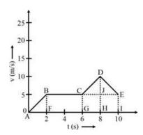
15. Given below is the velocity-time graph for the motion of the car. What does the nature of the graph show? Also, find the acceleration of the car.
