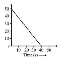
13. A car is moving on a straight road with uniform acceleration. The speed of the car varies with time as follows:
